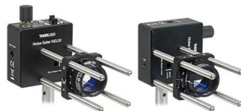
Click to Enlarge The Noise Eater can be post mounted in two different orientations to match the input light's direction of polarization. A CRM1T (/M) Cage Rotation Mount and four 30 mm Cage Rods can mount a half-wave plate for fine tuning the polarization alignment.
